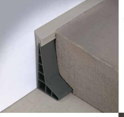
Along the perimeter there must necessarily be a sufficient dilatation space. Using the joint GC, plus the soft profile GCP you will get at one go both the required level on which to place the shafts, the necessary dilatation and a nice finish of the perimeter, avoiding need of further skirting.
